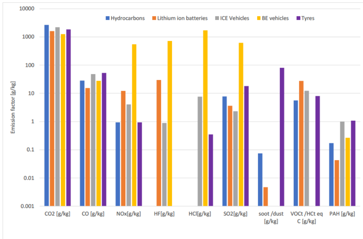
Figure 16: Emission factors for LIBs compared to other fuels.
